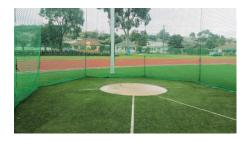
**Thor** cages are Cyclone 2 / Hurricane 1 wind rated and can remain erected and usable in most wind conditions. The gates have no frames and wheels which makes them easy to operate by one person. Vertical net retaining ropes are easily adjusted to keep the net in the correct playing position.
